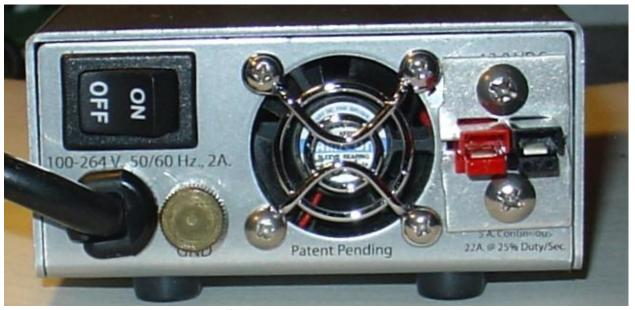
Figure 6: Completed PowerPole modification to the HPS-1a.
