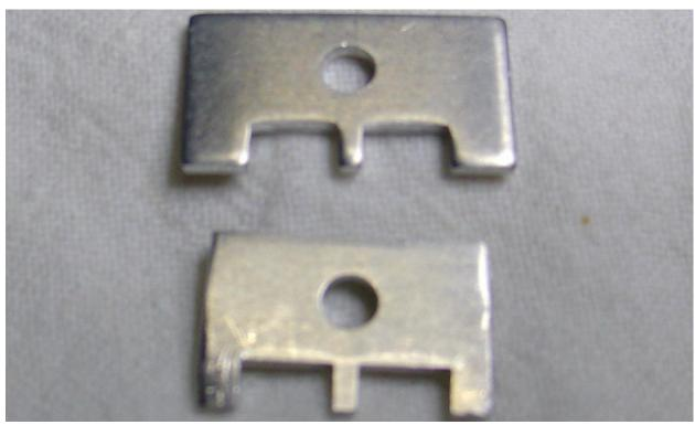
Figure 1: Upper clamp is unmodified. Lower clamp has had 0.1" nibbled from each side.
